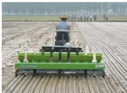
**Fig.2 Precision rice hill-drop drilling machine**
