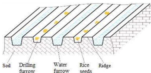
**Fig.1 Principle of precision rice hill-drop drilling technology**
